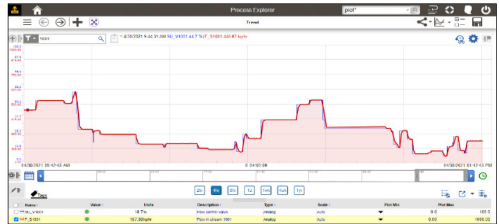
Time series trending of Aspen IP.21 data with many functions: zoom, annotations, comments, time shifting, control of pens and more.
